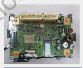
Place the board on the top of the metal case and reassemble the rest parts
